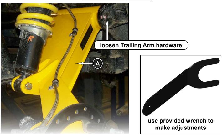
Trailing Arm, Passenger (A) shown off machine for clarity
