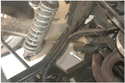
2. Use the included self tapping screws to secure the heat shield to the frame rail as indicated.
