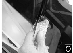
**Step 21:** Unlock latch and depress lever to open the latch. Carefully shut door, aligning the loose striker pin with the door latch and making sure the door does not collide with outside plastics. Due to the variances in the factory door opening, the rear mount and/or striker mount may need to be adjusted to allow the latch to properly catch.
