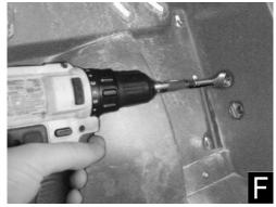
**Step 9:** Locate passenger side front door striker mount (Figure G) and striker mount hardware. Thread jam nut all the way on to striker pin and place a flat washer on to striker pin. Place striker pin onto mount and then secure the pin with flat washer and jam nut. Make jam nut finger tight for adjustment later on in the installation.
